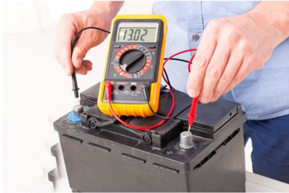
DC voltage reading
