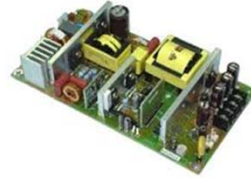
Low Voltage Power Supply
