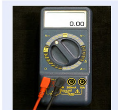
This image shows a switched range Multimeter: The central knob has lots of positions, and you must choose which one is appropriate for the measurement you want to make.
