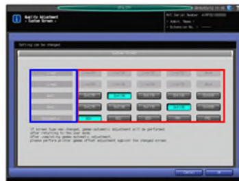
Default for each Custom Screen Line 1: Line 190 Line 2: Line 180 Dot 1: Dot 190 Dot 2: Dot 130 Stochastic: ED1
